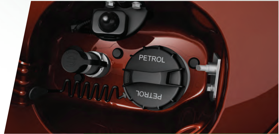
Micro Switch To Keep The Car Switched Off At Time Of Refueling
