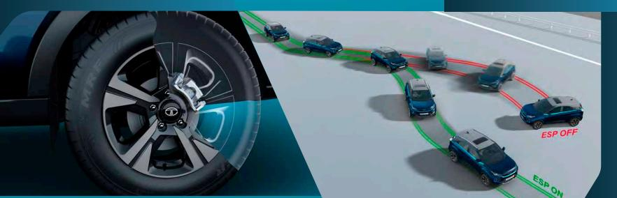
As you drive off to new destinations, the Nexon EV MAX's ESP® (Electronic Stability Program) helps keep you on course. It works with the innovative i-VBAC (Intelligent Vacuum-less Boost & Active Control) system to reduce stopping distances by improving brake dynamics.
