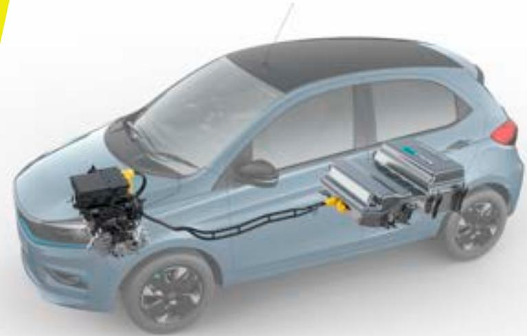
IP67 Certified Battery Pack and Motor
